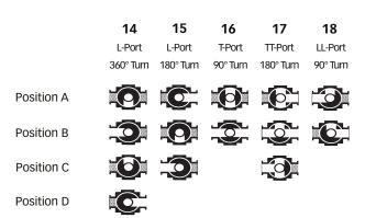
Fail position must be selected for spring return actuators only.
